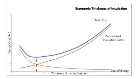
The generic graph above shows the energy cost, insulation cost, and total cost used to determine economic thickness for an insulated pipe.
