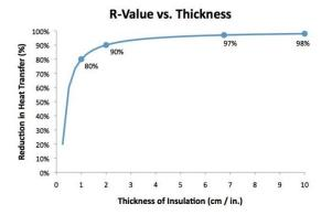
There is a substantial difference between insulation for temperature control and insulation for heat loss control. For instance, the graph (below) shows the heat loss control of the spray-in-place urethane foam insulation. Any insulation will have a similar graph but with thicker amounts of insulation. This graph points out that more insulation is not necessarily cost effective. There is a point where more insulation is pointless from a total heat loss perspective.
